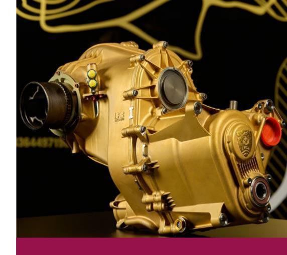
Ricardo has worked with Rodin Cars to develop a fully integrated gearbox solution for its FZERO, as well as a new transmission for its first electric car
